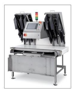
RAYCON D product inspection systems detect all contaminants that due to their density, chemical composition, or mechanical dimensions absorb X-radiation to a lesser or greater degree than the surrounding product. For example, metal, glass, ceramics, and stone contaminants in food. RAYCON D will also detect some plastics (e.g. PVC, rubber) as well as other product defects (e.g. cracks, trapped air). Desired "contaminants" (e.g. aluminium clips on sausage chubs) can be masked out.
