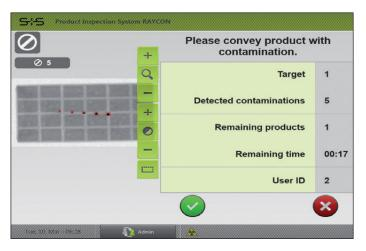
The product inspection system RAYCON D supports the operator actively in process control with the AuditCheck feature.
