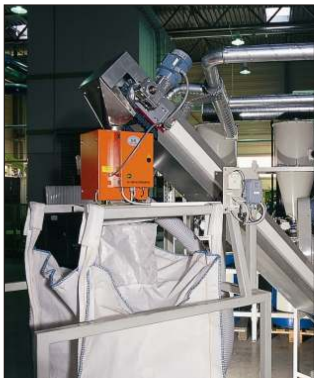
RAPID COMPACT metal separator employed for quality inspection in the process of filling into big bags
