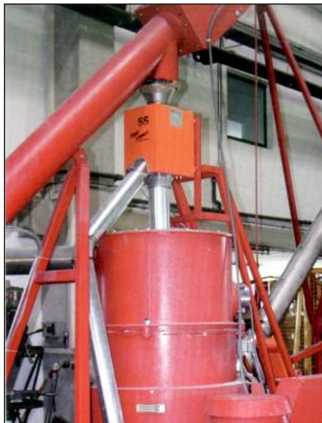
RAPID COMPACT metal separator employed for machine and mould protection before the pre-drier of an injection moulding machine
