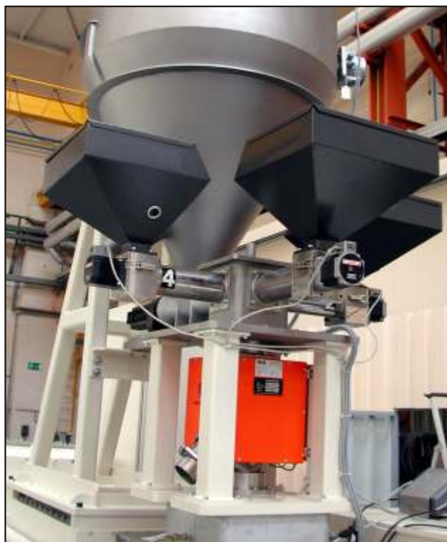
RAPID COMPACT metal separator installed before a twin screw extruder for the examination of PVC powder
